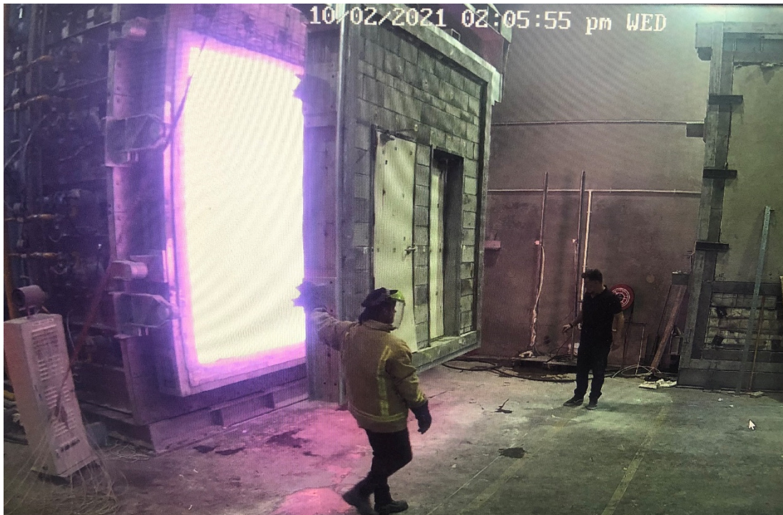
FDC Test Doors being removed from the Furnace after 4hours with Temperatures up to 1150°C – Still Very much intact
