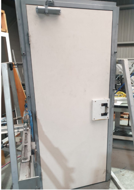
FDC Door Still in Perfect Condition after 100,000 slam cycles
