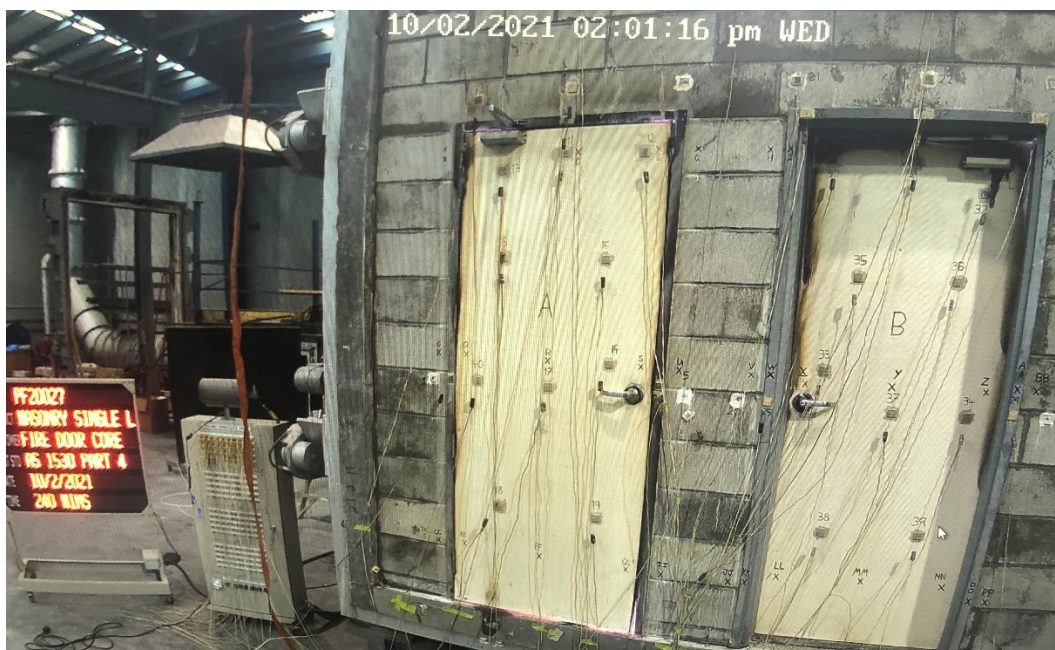
Unexposed Face of FDC Test Doors After 4hours without failure
